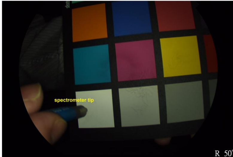
Figure 2. The spectra were collected utilizing a 24-color checker reference and a spectrometer (Ocean Optics, QE65000), with simultaneous measurements of the light source spectrum.
