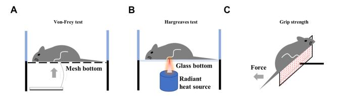
Supplementary Figure 2. The schematic diagram of the apparatus used in performing pain-associated behavioral experiment. (A) Von-Frey test, (B) Hargreaves test, and (C) Grip strength.
